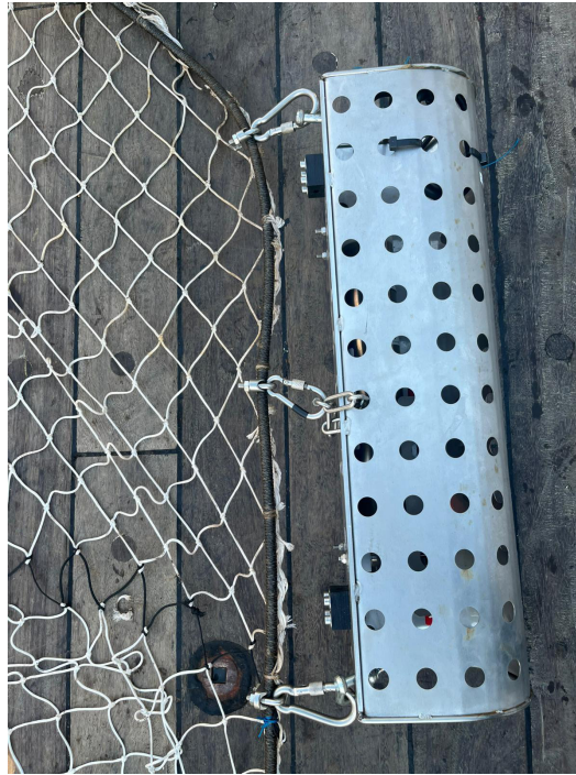
Figure 4. CTD cage (SBE37SM) attached to the float rope (headline) of the GOC73 trawl net using stainless steel clamps and a locking carabiner. Photo: ICATMAR / MEDITS-AUT25.
