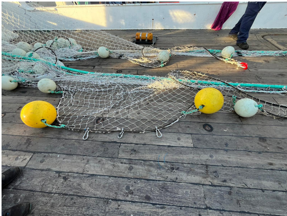
Figure 5. Detail of the 20-litre buoyancy spheres mounted on the cage frame to achieve near-neutral buoyancy during deployment. Photo: ICATMAR / MEDITS-AUT25.
