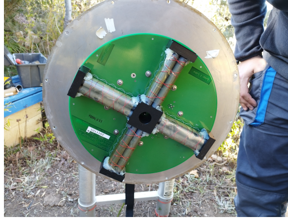
Figure 3: Cross-loop antenna board from a CODAR 13.5 MHz station. Image provided by Qualitas Remos SL.
