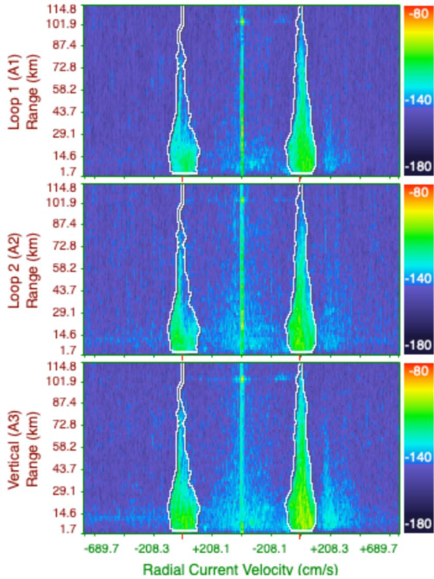
Figure 7: Spectra loop example of XarxaHFCat radar CSQ showing the spectra of the three radars that compose a single CODAR.
