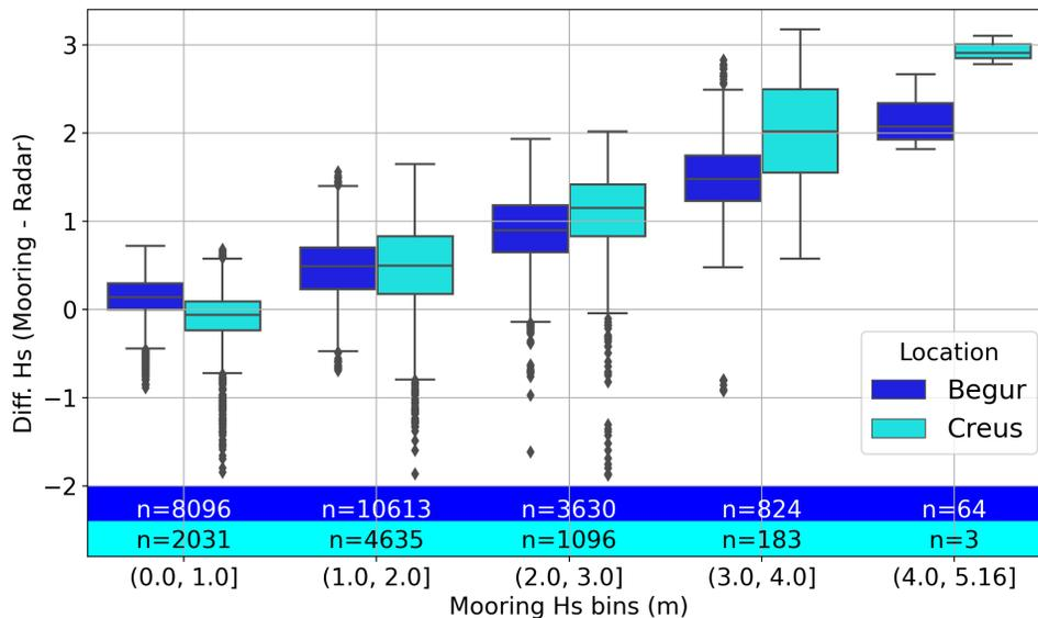
Figure 3: Boxplot of difference  $H_s$  measured by the buoy and the HF radar binned by  $H_s$  magnitude using mooring buoy as a reference in Begur,  $n$  is the number of observations.
