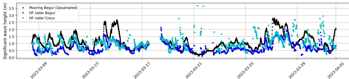
Figure 6: Comparison of significant wave height ( $H_s$ ) data in Begur: mooring buoy ( $\blacktriangle$ ) versus radar data from Begur ( $\bullet$ ) and Creus ( $\blacksquare$ ), unfiltered data.
