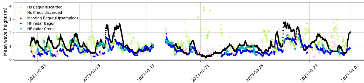
Figure 2: Comparison of significant wave height ( $H_s$ ) data in Begur: mooring buoy ( $\blacktriangle$ ) versus radar data from Begur ( $\bullet$ ) and Creus ( $\blacksquare$ ), with discarded Begur ( $\ast$ ) and Creus ( $\ast$ ) data.
