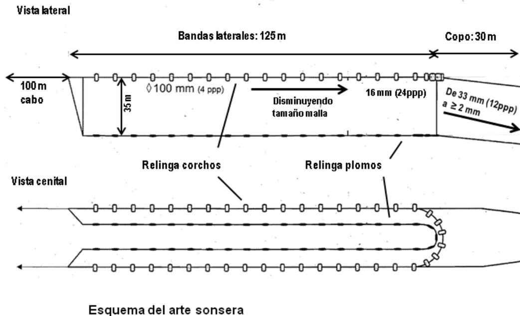
Figure 4.1.1. Drawing of the boat seine “sonsera” characteristics.
